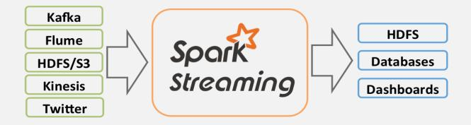
Internally, Spark Streaming receives live input data streams and divides the data into batches, which are then processed by the Spark engine to generate the final stream of results in batches.
